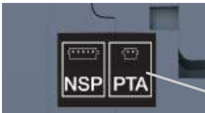
Integrated PTA output contact Output contact dedicated to the overload prealarm.
